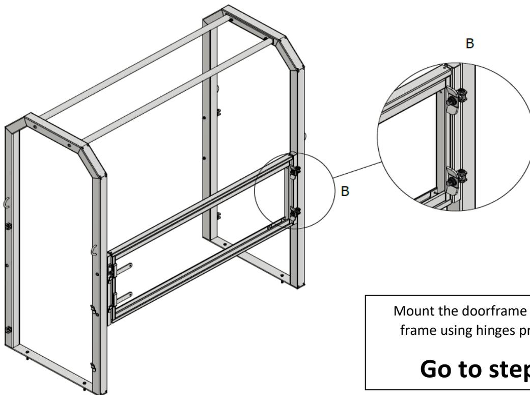
Mount the doorframe onto the frame using hinges provided.
