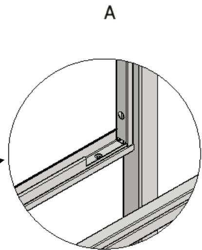
Make sure you don't install the extra plate until you have placed the planks. (Last step)
