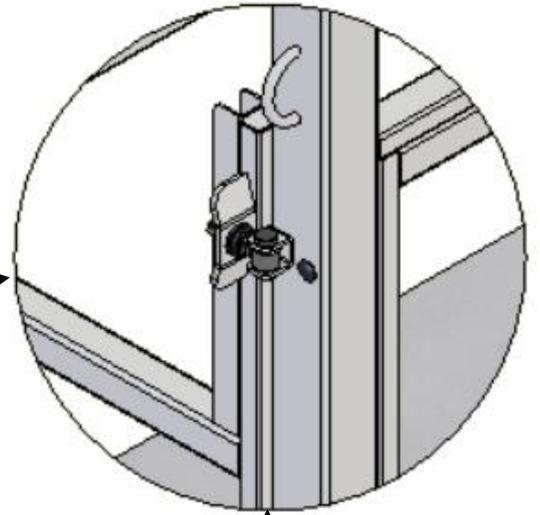
Mount the doorframe onto the frame using hinges provided.
