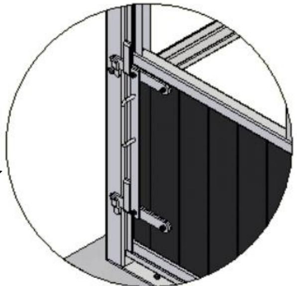
Mount the parallel lock onto the frame using the set of bolts provided and install the planks.
