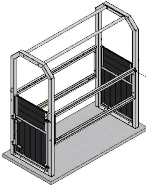
Place the planks on top of the doorframe.
