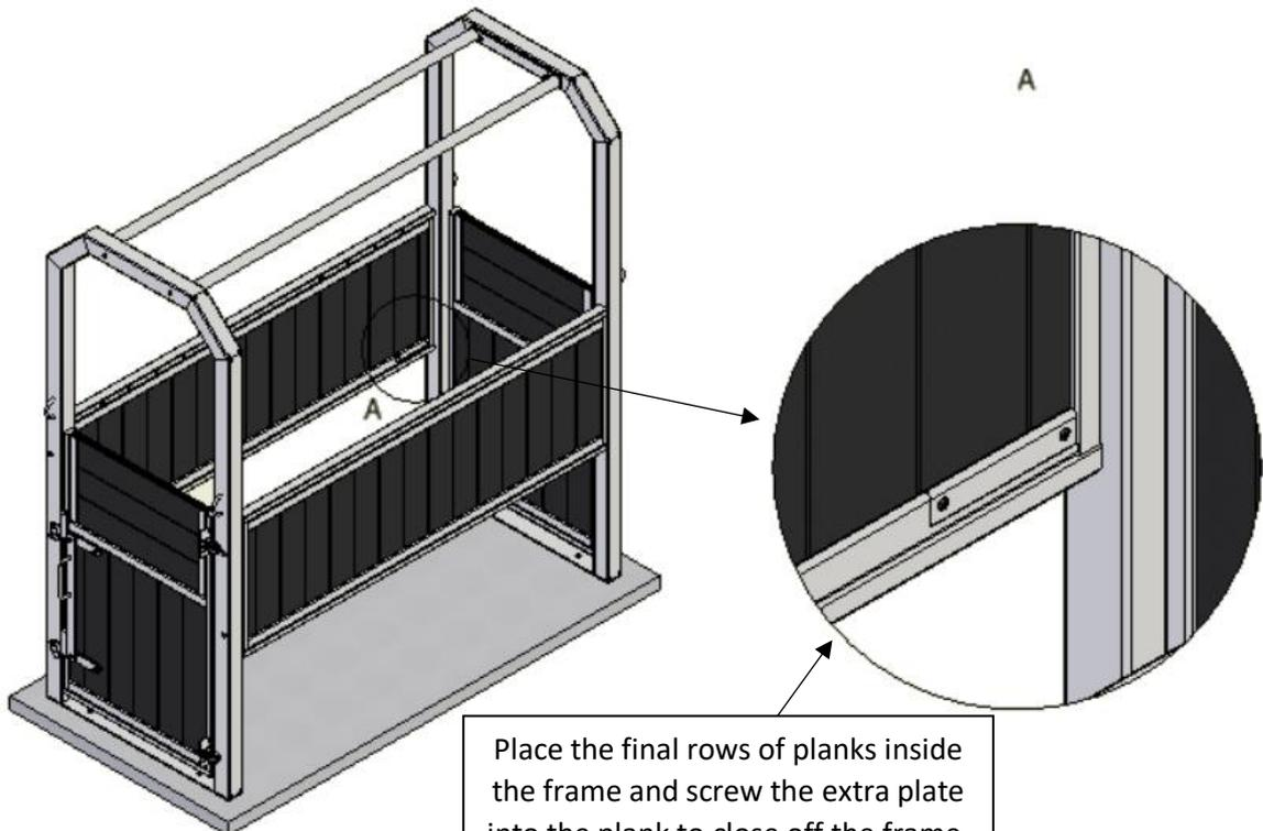
Place the final rows of planks inside the frame and screw the extra plate into the plank to close off the frame.
